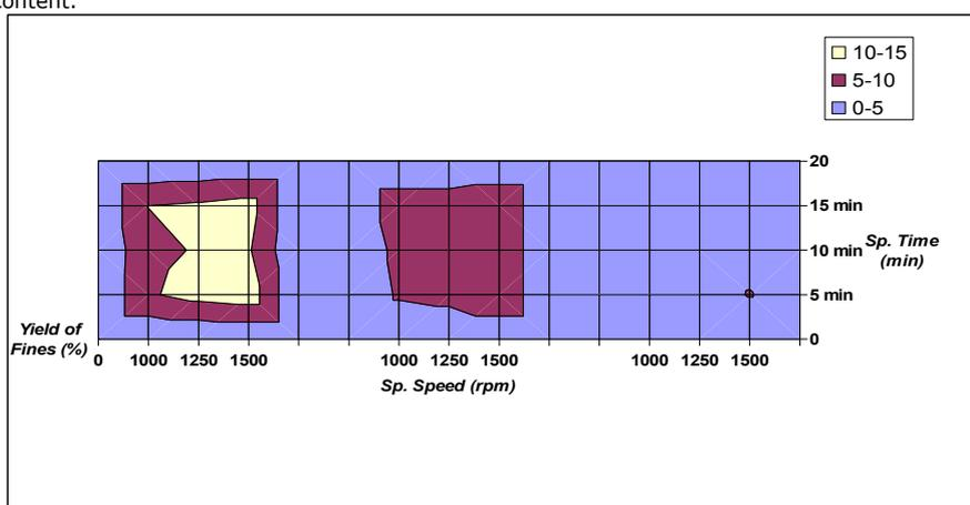
Figure 2a. Surface representation of results from factorial experiments for the yield of fines (%) as a function of speed/water content.
