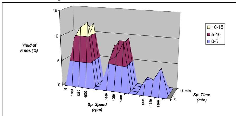
Figure 2b. Three-D representation of results from factorial experiments for the yield of fines (%) as a function of speed/water content.
