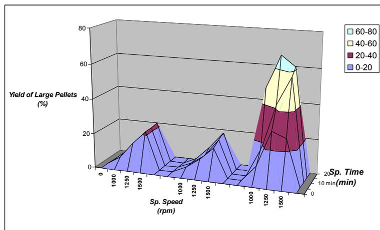
Figure 3b. Three-D representation of results from factorial experiments for the yield of Large Pellets (%) as a function of speed/water content.
