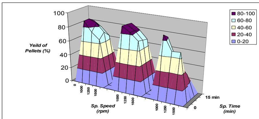
Figure 1b. Three-D representation of results from factorial experiments for the yield of pellets (%) as a function of speed/water content.
