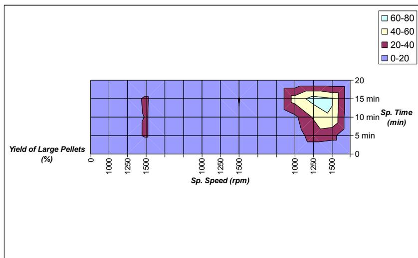
Figure 3a. Surface representation of results from factorial experiments for the yield of Large Pellets (%) as a function of speed/water content.
